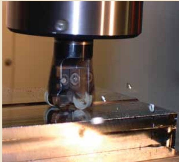
Hard Milling 55 Rc steel with Greenleaf's WG-300® whisker-reinforced ceramic inserts.
