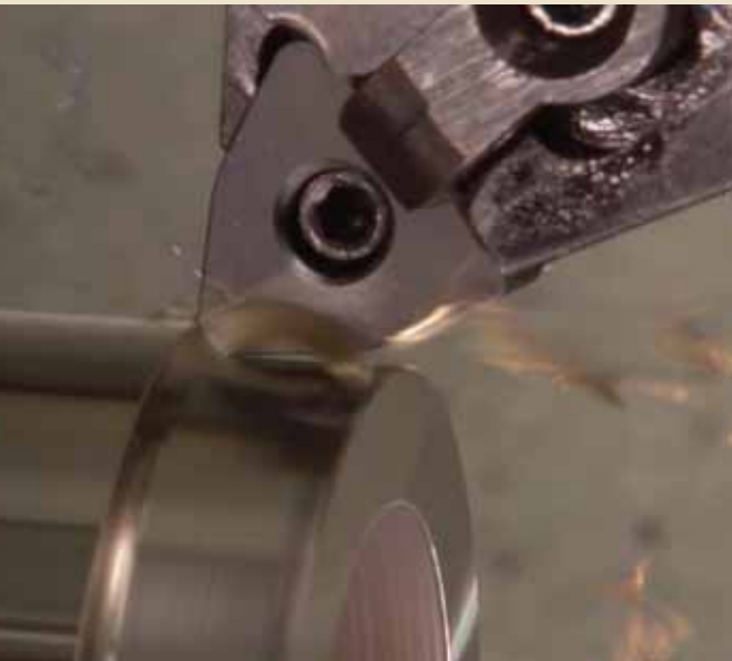
A Greenleaf whisker-reinforced, ceramic insert turning hardened steel.
